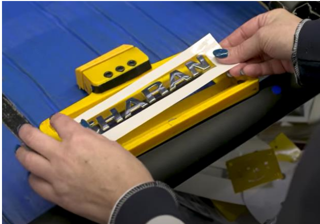
Figure 6. AM-Produced Fixtures and Worker Assistive Tools
