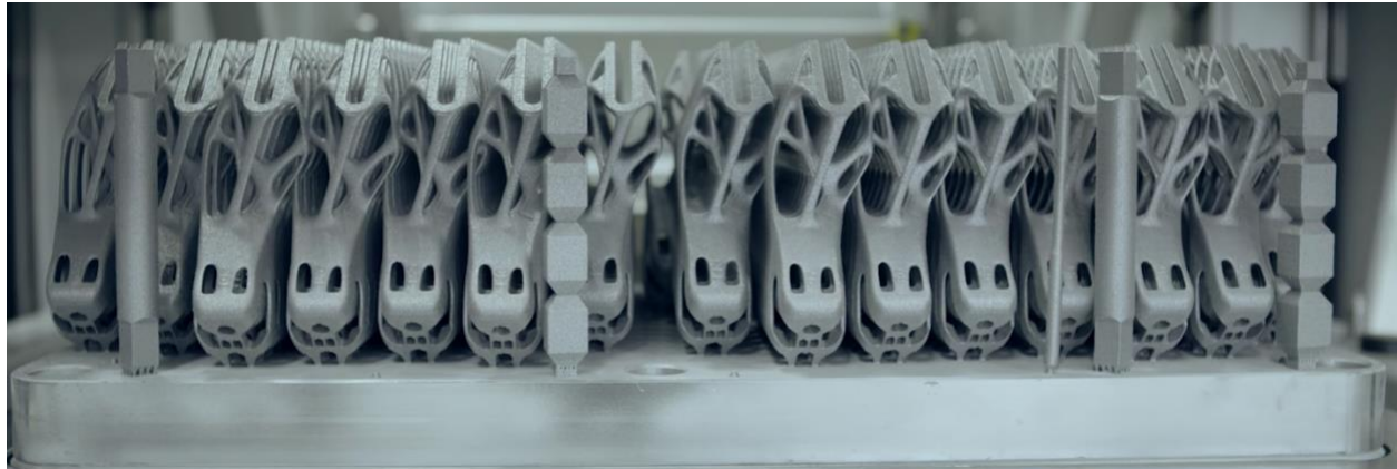
Figure 9. Hinge brackets for the BMW i8 Roadster are arrayed on a build platform after printing has concluded.
