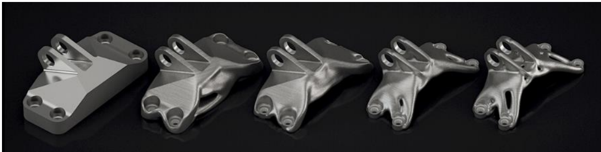
Figure 5. This rendering of a generative design workflow contrasts a conventionally machined bracket (far left) with iterative improvements in material placement resulting in a shape-optimized, additively manufacturing bracket (far right).
